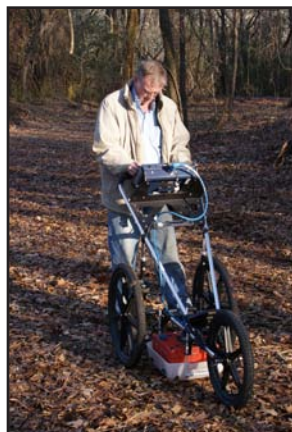
(Left) Annual walk commemorating the role of Tuscumbia Landing in the Trail of Tears, here led by 90 year-old Chickasaw elder Flora Perry. (Center) Ground-penetrating radar used to image subsurface features of historical significance. (Right) Image produced from ground-penetrating radar and GPS data. (Photos courtesy of Marty King)
